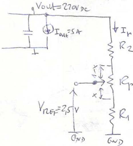
$$I_r = \frac{220 \text{ V}}{R_2 + R_p + R_1}$$
