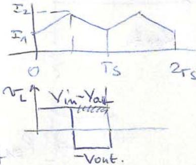
$$L(I_2 - I_1) = (V_{in} - V_{out}) \cdot t_{on} = (V_{in} - V_{out}) \delta T$$
