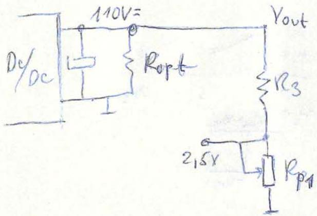
$$\frac{V_{out}}{R_{p1} + R_3} \cdot R_{p1} = V_{ref}$$
