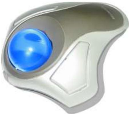
Used as an alternative to a mouse. To operate it the user rotates the ball which moves the pointer on screen. They are particularly easy to use for those with limited movement in their hands and are often used in Computer Aided Design (CAD) for their increased precision over a mouse.
