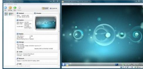
Screenshot of VirtualBox v4.1.8 running a copy of Ubuntu 11.04 on Windows 7. The window to the left is VirtualBox virtual machine manager and the one to the right is the desktop of Ubuntu
