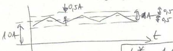
$$I_{L_{max}} = I_{L_{out}} + \frac{\Delta i_L}{2} = 10 \text{ A} + \frac{1}{2} \text{ A}$$
