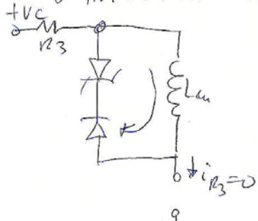
$$L_m \cdot \Delta i = V' \cdot t_{on} \Rightarrow \Delta i = \overline{i}_{L_m} = \frac{V' \cdot t_{on}}{L_m}$$
