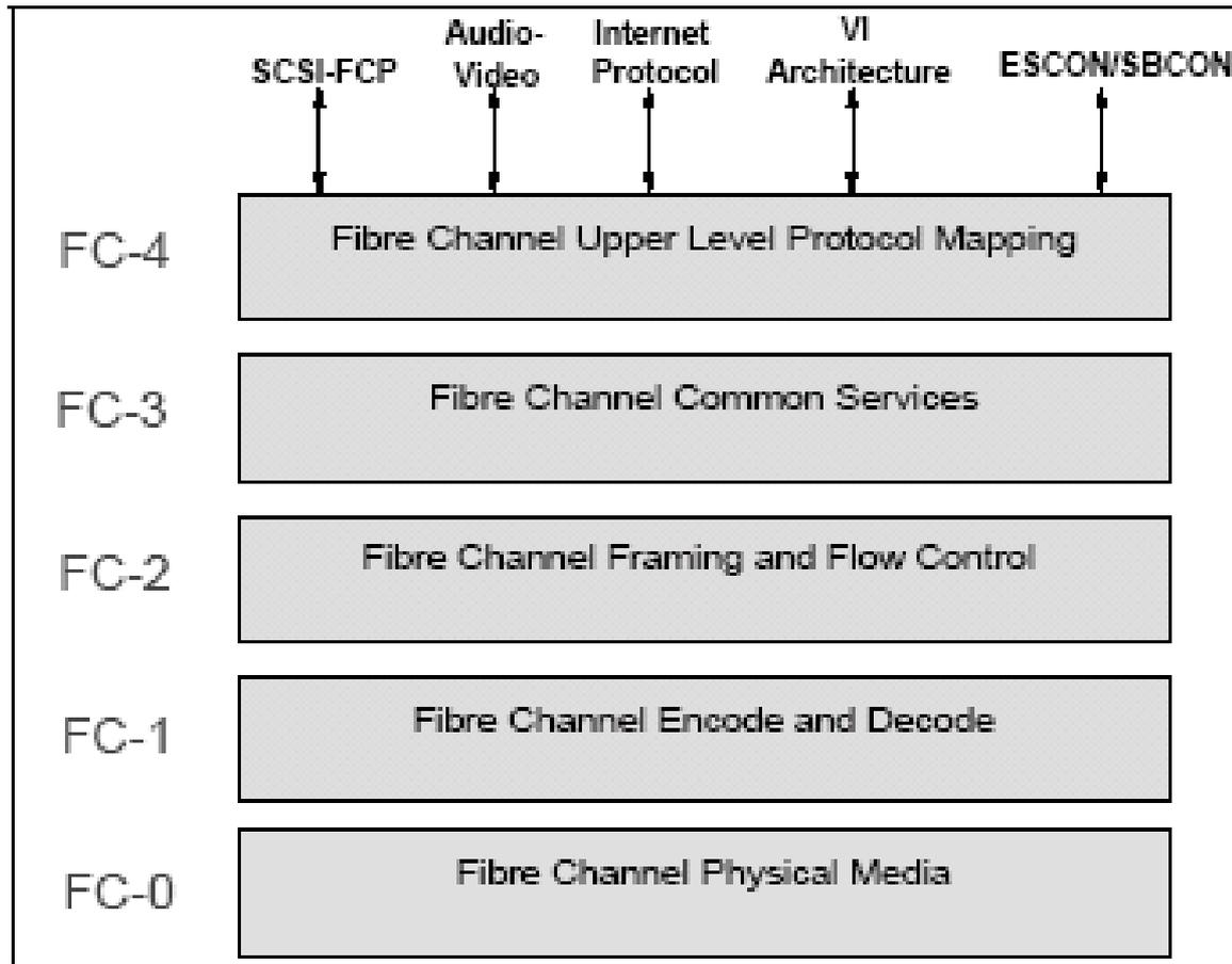
Figure 3-30 Fibre Channel layers
