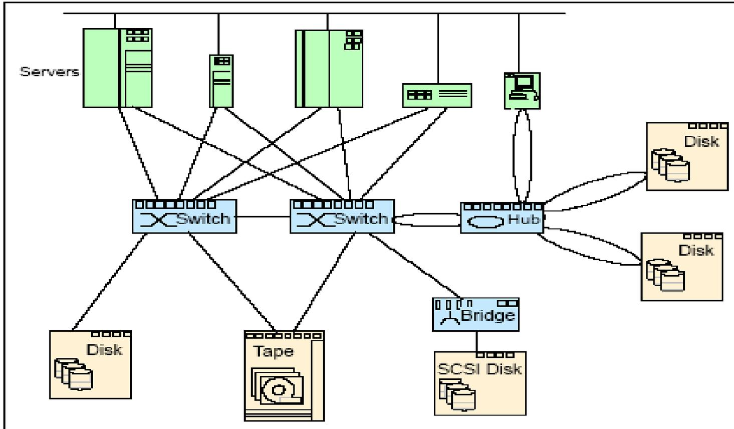
Figure 3-8 Sample switched fabric configuration
