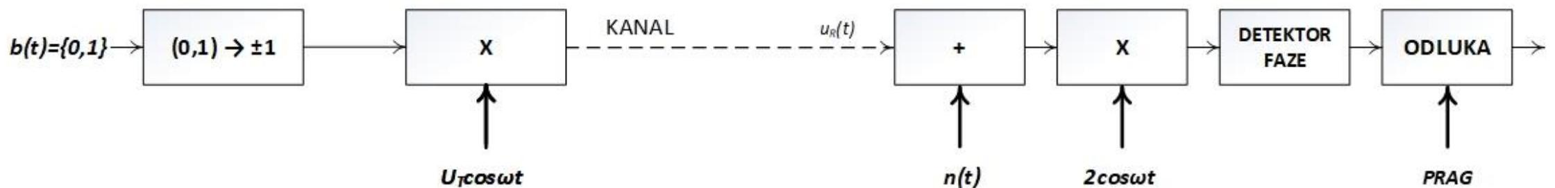
$$u_R(t) = b(t)U_T \cos \omega t, \quad b(t) \in \{\pm 1\}$$
