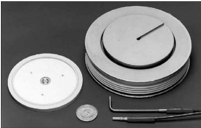
FIGURE 24.24 Silicon wafer and construction of the LTT. The light guides appear in the bottom right-hand corner of the photo.
